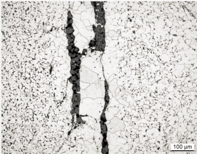
Fig. 9: Micrograph of cross-section from Fig. 3 (detail), nital etched, bright field. We observe a hypoeutectoid steel including a ferritic zone surrounded by slag inclusions,
