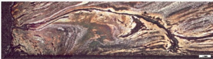
Fig. 6: Micrograph of the metal sample from Fig. 3 (reversed picture, detail), etched with Oberhoffer's reagent, bright field. The etching shows the P segregation near the welding line and outlines the irregular P distribution in the metal (white P-rich areas, dark P-poor areas),
