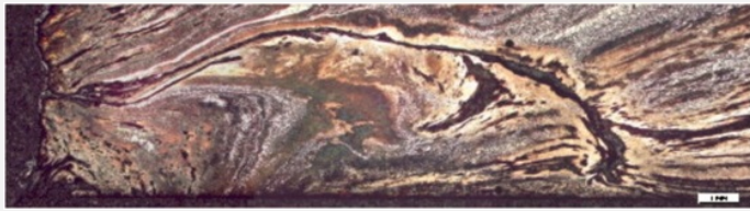
Fig. 6: Micrograph of the metal sample from Fig. 3 (reversed picture, detail), etched with Oberhoffer's reagent, bright field. The etching shows the P segregation near the welding line and outlines the irregular P distribution in the metal (white P-rich areas, dark P-poor areas),
