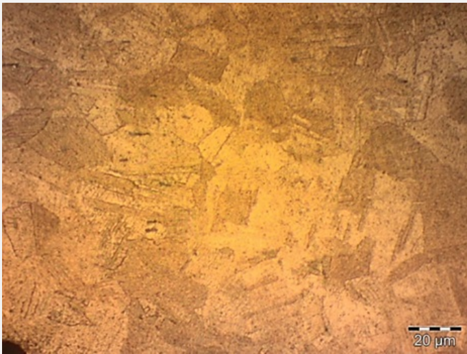
Fig. 9: Micrograph of the selected area of Fig. 8, etched, bright field, 500x. The grains show both twin and strain lines,
