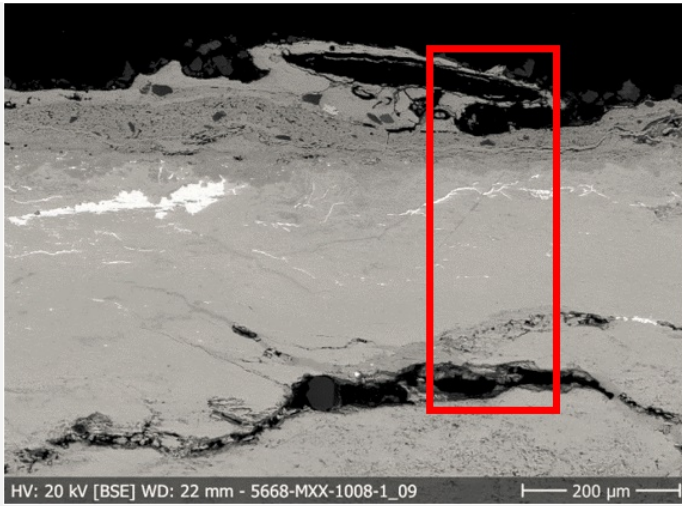
Fig. 11: SEM image of the cross-section from Fig. 10 (detail), BSE-mode. The mapped area (Fig. 12) is marked by a rectangle,
