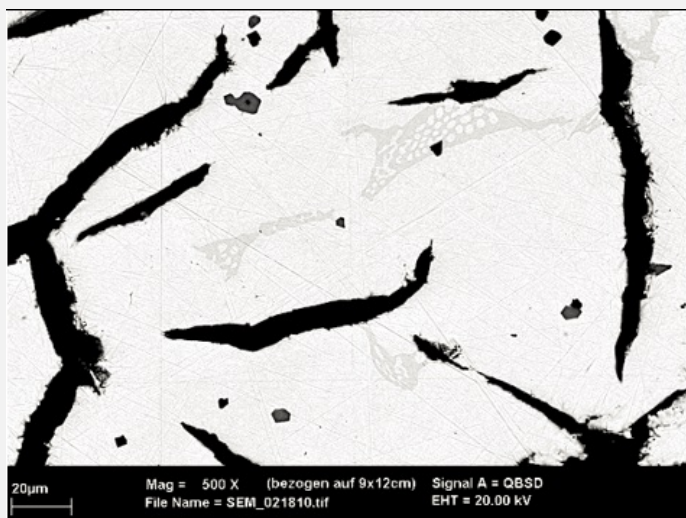
Fig. 6: SEM image from Fig. 3 (detail), BSE-mode, unetched. We observe the graphite flakes in black, the manganese sulphide inclusions in grey and the eutectic mixture in light-grey,
