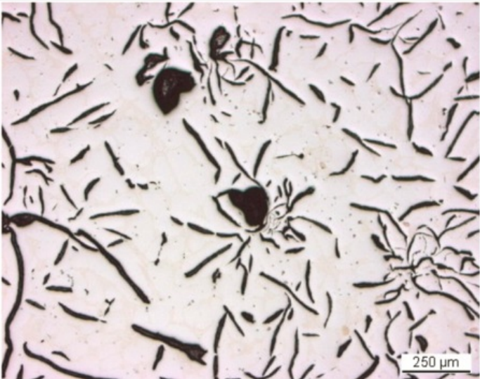
Fig. 5: Micrograph of the metal sample from Fig. 3 (inverted picture, detail), unetched, bright field. We observe graphite flakes and irregular nodules in black and the metal in white. The small grey spots are manganese sulphide inclusions,
