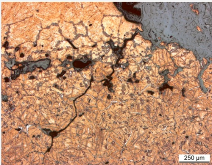
Fig. 6: Micrograph of the metal sample, detail from Fig. 5, etched, bright field. We observe martensite (in orange), cementite (in grey), porosity and intergranular cracks (in black) and corrosion,
