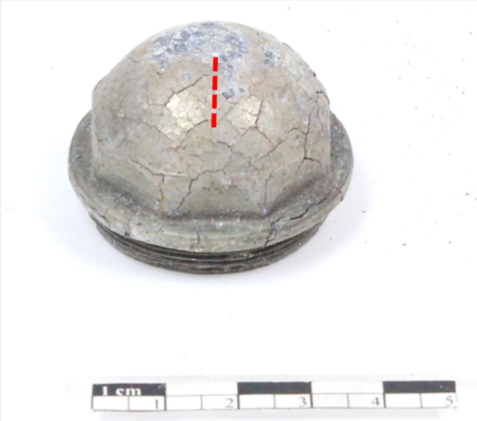
Fig. 2: Zones of the artefact submitted to visual observation and location of sampling area (a cross-section of the metal marked by the stippled line),
