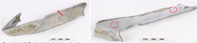
Fig. 2: Location of sampling area (a cross-section through the metal marked by the stippled line) and of powder samples (red circles),
