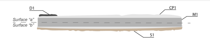
Fig. 3: Schematic presentation of the artefact (a cross-section of the metal) based on visual macroscopic observation. CP = corrosion product, D = deposit, M = metal, S = soil,
