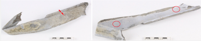
Fig. 2: Location of sampling area (a cross-section through the metal marked by the stippled line) and of powder samples (red circles),
