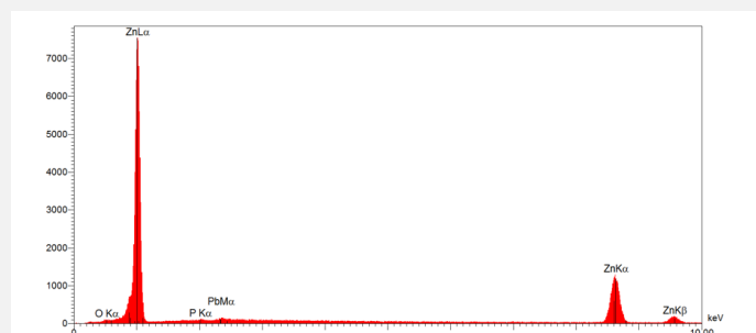
Fig. 6: Chemical composition of the metal. Method of analysis: SEM-EDS. Lab. of Electronic Microscopy and Microanalysis, Néode, HEI Arc,
