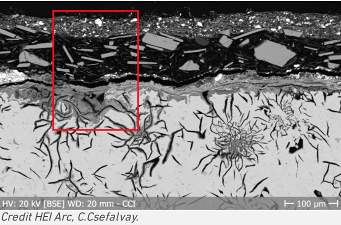
Fig. 11: SEM-image (BSE-mode) of the selected area in Fig. 10 (detail), showing the morphology of the paint layers and the area selected for elemental mapping (Fig. 12),
