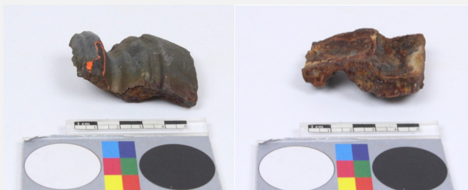
Fig. 1: Cast iron fragment with paint coating; exterior (coated) surface and the rear (non-coated) surface to the left and right, respectively,
