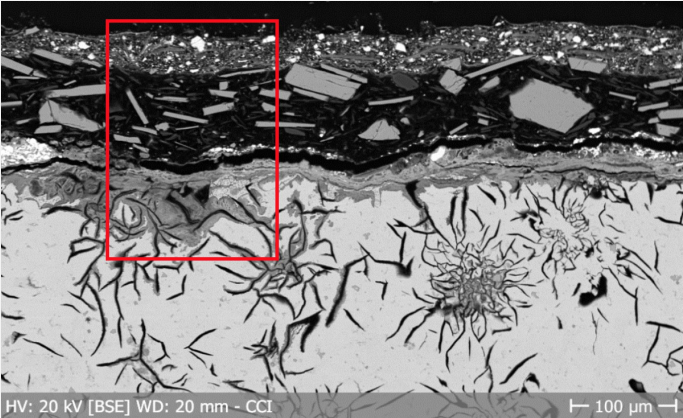
Fig. 11: SEM-image (BSE-mode) of the selected area in Fig. 10 (detail), showing the morphology of the paint layers and the area selected for elemental mapping (Fig. 12),
