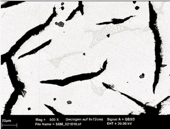
Fig. 6: SEM image from Fig. 3 (detail), BSE-mode, unetched. We observe the graphite flakes in black, the manganese sulphide inclusions in grey and the eutectic mixture in light-grey,
