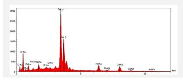
Fig, 12: EDS spectrum of sample 1 (yellow powder),
