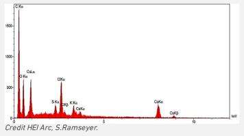
Fig. 16: EDS spectrum of sample 4 (white particle),
