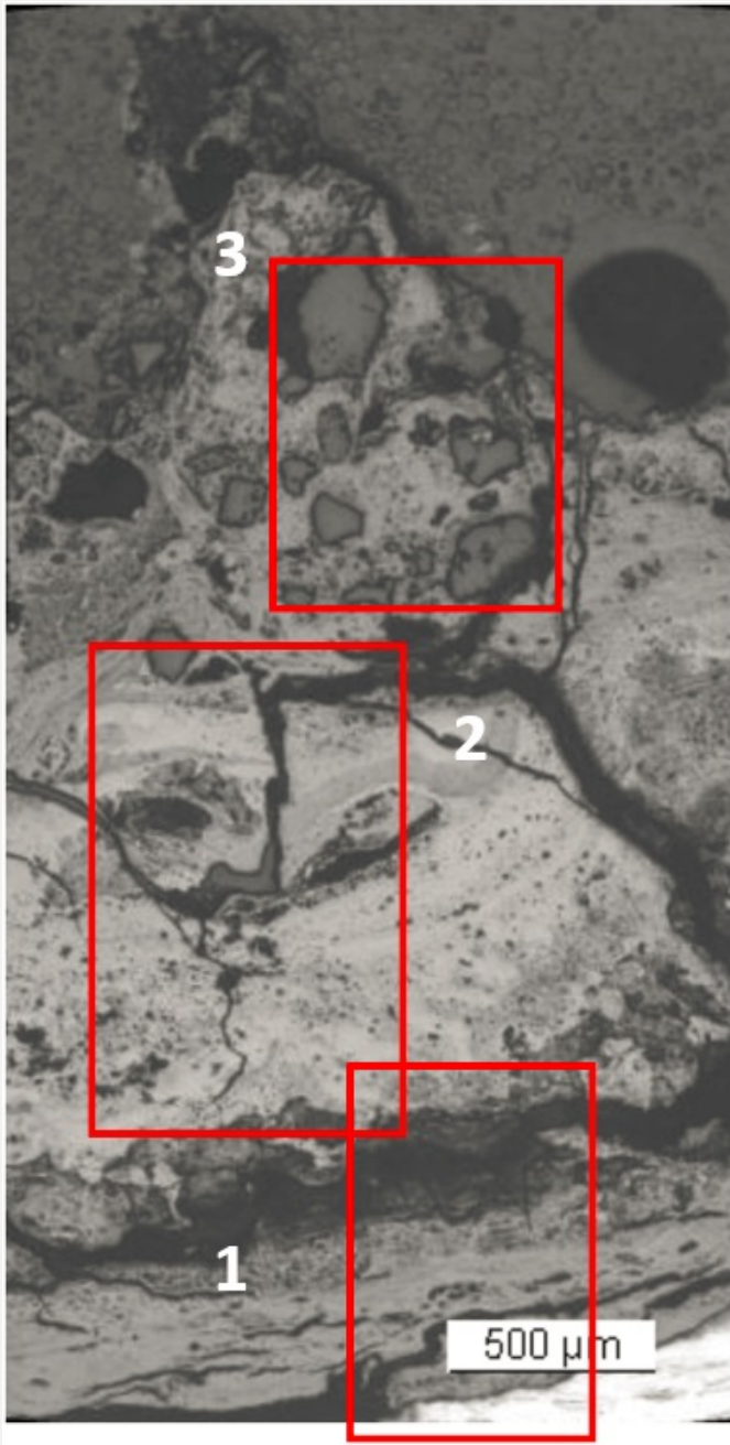
Fig. 7: Micrograph of the corrosion layer from Fig. 3 showing the metal - corrosion crust interface (detail, rotated by 45°) and corresponding to the stratigraphy of Fig. 4, unetched, bright field. Areas 1 (inner layer, CP3) to 3 (outer layer, CP1) are indicated,
