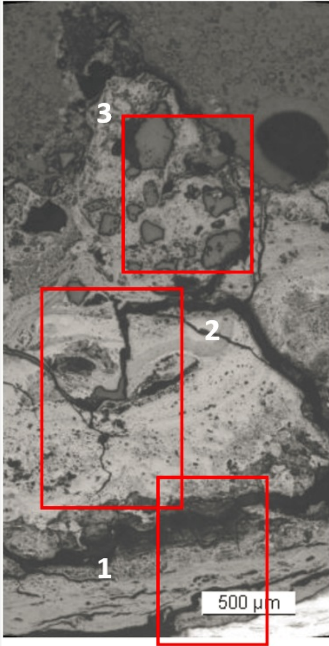
Fig. 7: Micrograph of the corrosion layer from Fig. 3 showing the metal - corrosion crust interface (detail, rotated by 45°) and corresponding to the stratigraphy of Fig. 4, unetched, bright field. Areas 1 (inner layer, CP3) to 3 (outer layer, CP1) are indicated,
