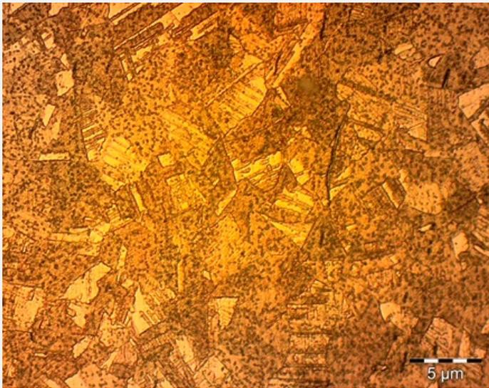
Fig. 8: Micrograph of the metal sample from Fig. 4, etched, bright field, 50x. Polygonal and twinned grains with strain lines are observed. The dotted surface is the result of over-etching,
