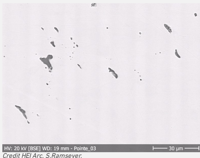
Fig. 8: SEM, BSE-mode picture of inclusions in remaining metal,
