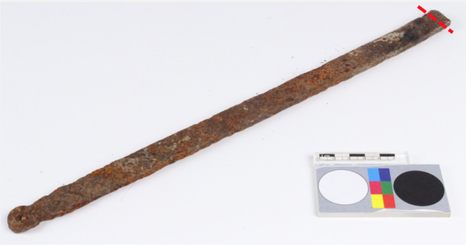
Fig. 2: Zones of the artefact submitted to visual observation and location of sampling area (a cross-section of the metal, marked by a stippled line),
