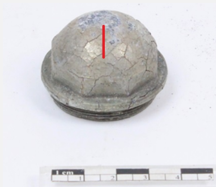
Fig. 2: Zone of the artefact submitted to visual observation and location of sampling area (a cross-section of the metal marked by the red line),
