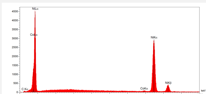
Fig. 8: EDS-spectrum showing the chemical composition of the metal plating (M1). Method of analysis: SEM-EDS. Lab. of Electronic Microscopy and and Microanalysis, Néode, HEI Arc,
