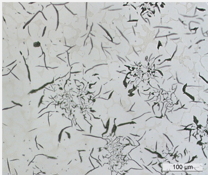
Fig. 8: Micrograph of the metal sample from Fig. 4 (detail), unetched, bright field. The microstructure of the metal consists of graphite flakes in a matrix of dendrites (light grey) and an interdendritic eutectoid phase (light brown). The global analysis of the metal (Fig. 9) was carried out on a surface area of similar size,
