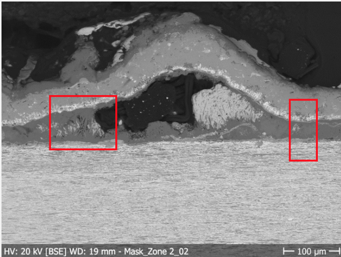
Fig. 7: SEM image (BSE-mode) of the metal sample from Fig. 4 with detail (Fig. 8) indicated by the left red rectangle. The selected area for elemental chemical distribution (Fig. 9) is marked by the right red rectangle,
