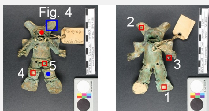
Fig. 2: Bat figure, front (left) and back (right) view with location of XRF analyses (red squares), FTIR analysis with sampling (blue point) and SEM-EDS analysis (red point),
