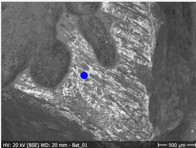
Figs. 8: SEM images of the metal on the nose of the bat. The blue point represents the area for the EDS point analysis (Fig. 9),
