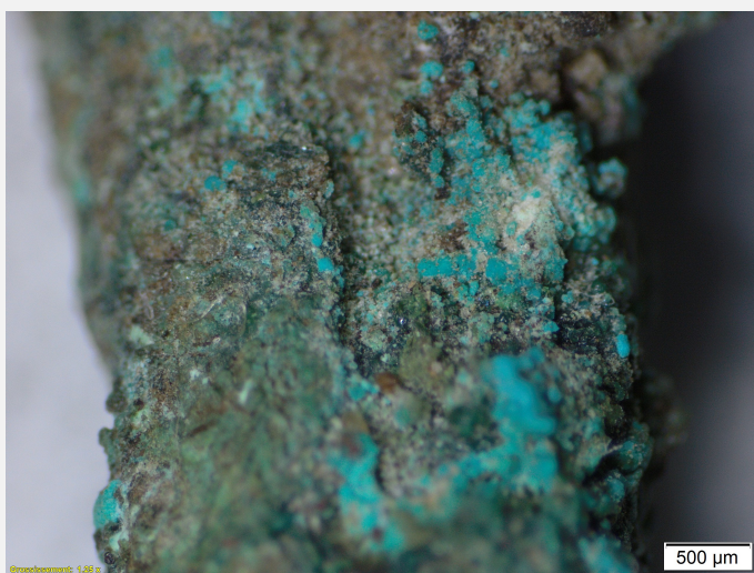
Fig. 6: Detail of Fig. 4 with blue corrosion products in cluster, sample 2 (CP4)
