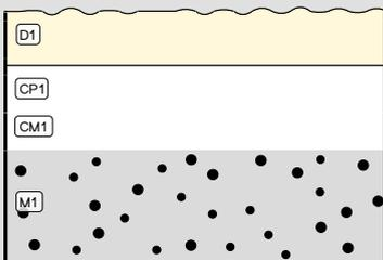
Fig. 4: Stratigraphic representation of the sample taken from the front fastening plate in cross-section using the MiCorr application. The characteristics of the strata are only accessible by clicking on the drawing that redirects you to the search tool by stratigraphy representation. This representation can be compared to Fig. 8, Credit HE-Arc CR.
