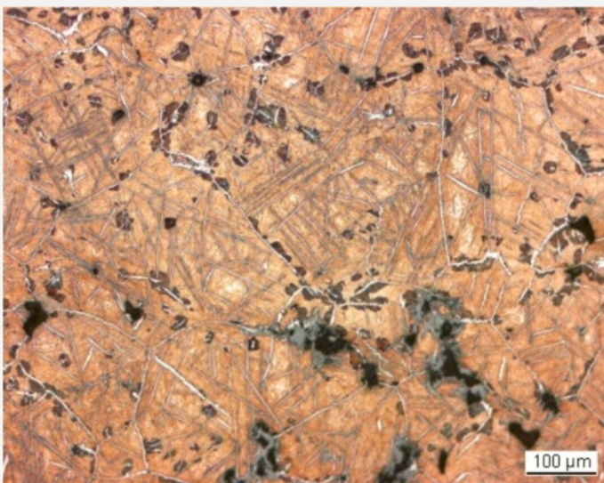
Fig. 9: Micrograph of the metal sample, detail from Fig. 5, etched, bright field. Hypereutectoid steel with a structure of cementite in white in the grain boundaries and in needle form combined with martensite (pink). Some bainite occurs around the grain boundaries,
