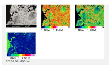
Corrosion form Uniform - intergranular
