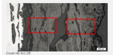
Fig. 11: Micrograph showing the metal - corrosion crust interface from Fig. 3 (reversed picture, detail), unetched, bright field. The areas selected for elemental chemical distributions (Fig. 13 (left) and Fig. 14 (right)) are marked by red rectangles,
