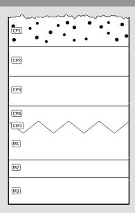
Fig. 4: Stratigraphic representation of sample 2 from the moil chisel in cross-section using the MiCorr application. The characteristics of the strata are only accessible by clicking on the drawing that redirects you to the search tool by stratigraphy representation. This representation can be compared to Fig. 12, Credit HE-Arc CR.
