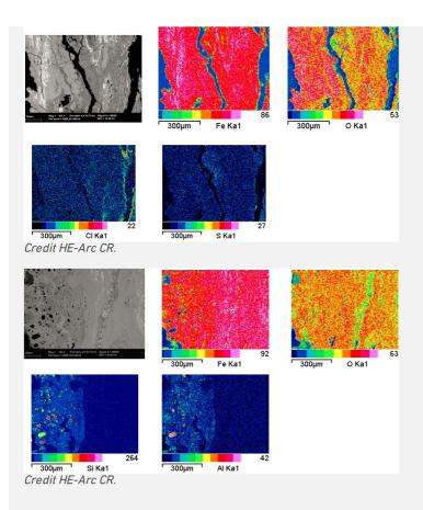
Fig. 14: SEM image, BSE-mode, and elemental chemical distribution of the selected area from Fig. 11 (reversed picture). Method of examination: SEM/EDS, Laboratory of Analytical Chemistry, Empa,
