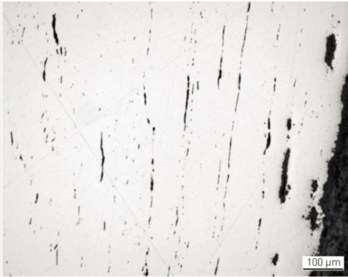
Fig. 5: Micrograph of metal sample 1 from Fig. 3 (reversed picture, detail), unetched, bright field. Slag inclusions organized in rows mark the welding seams,
