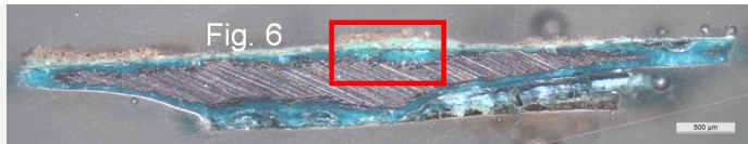
Fig. 4: Micrograph of the cross-section of the sample taken from the detached fragment of the situla showing the location of Fig. 6. Unetched, dark field, 50x,
