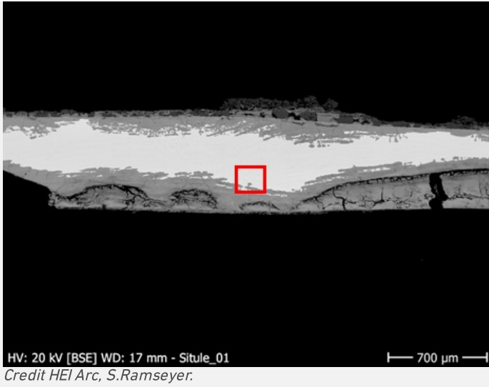
Fig. 7: SEM image, BSE-mode, of the metal sample from Fig. 4. Area of Fig. 8 is marked by a red square,
