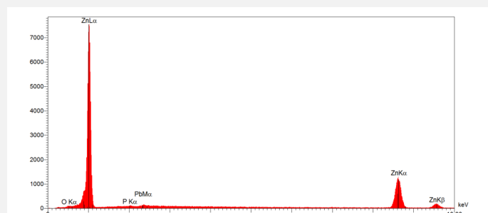
Fig. 6: Chemical composition of the metal. Method of analysis: SEM-EDS. Lab. of Electronic Microscopy and Microanalysis, Néode, HEI Arc,
