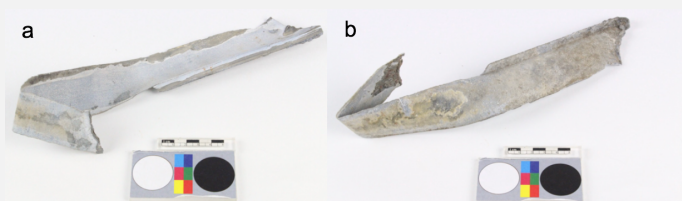
Fig. 1: Roof gutter element having different appearances on each of its surfaces: "a" on the left and "b" on the right,
