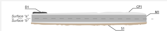
Fig. 3: Schematic presentation of the artefact (a cross-section of the metal) based on visual macroscopic observation. CP = corrosion product, D = deposit, M = metal, S = soil,
