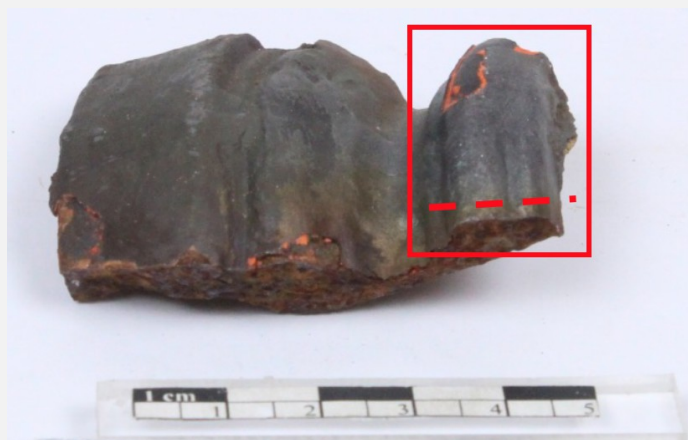
Fig. 2: Zone of the artefact submitted to visual observation (red square) and location of sampling (a cross section through metal including a few layers of paint, marked by the stippled line),
