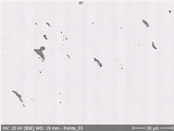
Fig. 8: SEM, BSE-mode picture of inclusions in remaining metal,
