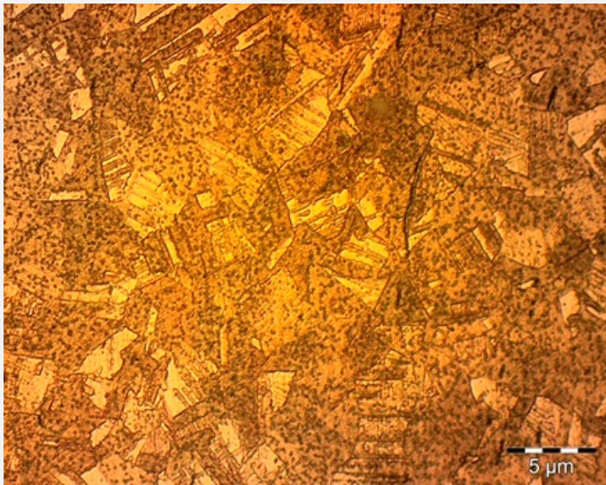
Fig. 8: Micrograph of the metal sample from Fig. 4, etched, bright field, 50x. Polygonal and twinned grains with strain lines are observed. The dotted surface is the result of over-etching,
