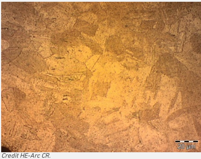
Fig. 9: Micrograph of the selected area of Fig. 8, etched, bright field, 500x. The grains show both twin and strain lines,
