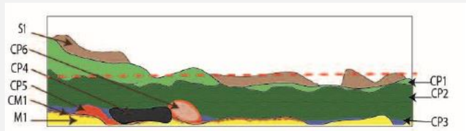
Fig 21 : Improved representation of the stratigraphy of corrosion layers of the bracelet from visual observations and analyses.
