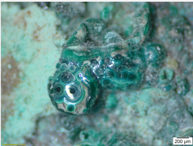
Fig. 7: Detail of Fig. 4 with green corrosion product, with eye-like structure, sample 3 (CP3)
