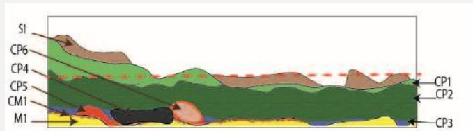
Fig 21 : Improved representation of the stratigraphy of corrosion layers of the bracelet from visual observations and analyses.
