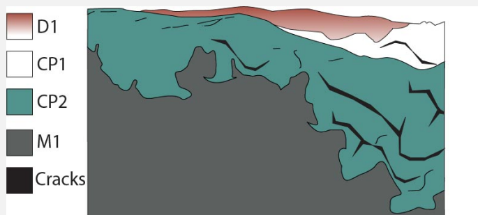
Fig. 6: Stratigraphic representation of the corroded exit pipe of the water pump in cross-section by macroscopic observation, M = metal, CP = corrosion product, D = deposit,
