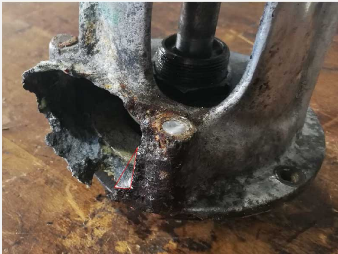
Fig. 5: Close-up view of the corroded exit pipe of the disassembled Hispano water pump, showing the sampled area,
