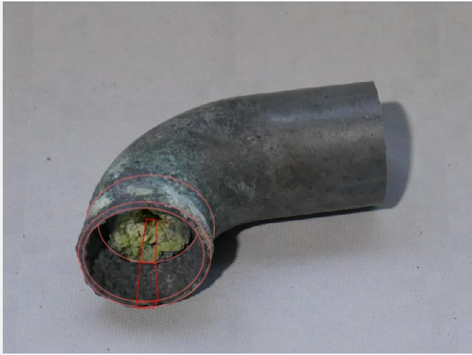
Fig. 3: Heavily corroded side of the Bugatti water pipe showing the sampling area indicated in red,
