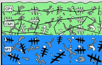
Fig. 7: Stratigraphic representation of the sample taken from the Bugatti water pipe in cross-section (dark field) using the MiCorr application. The characteristics of the strata are only accessible by clicking on the drawing that redirects you to the search tool by stratigraphy representation. This representation can be compared to Fig. 8 and 9, Credit HE-Arc CR, E.Granget.
