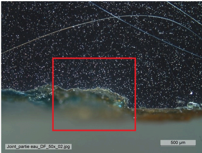
Fig. 10: Micrograph of the cross-section of the gasket, zone 2, shown on Fig. 5 unetched, dark field, showing the location of the SEM image of Fig. 11 (in red),
