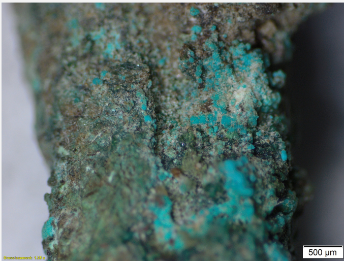
Fig. 6: Detail of Fig. 4 with blue corrosion products in cluster, sample 2 (CP4)
