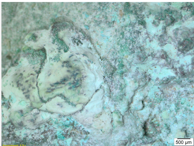
Fig. 5: Detail of Fig. 4 with whitish and not very cohesive corrosion product, sample 1 (CP1),
