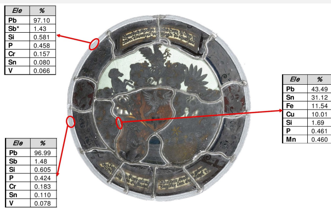
Fig. 2: XRF analysis of the different lead came of the "Stokar" stained glass panel. Tin (Sn) content is very variable from one came to another. Those with a very low Sn but a high Sb (1.4%) contents are much more corroded,
