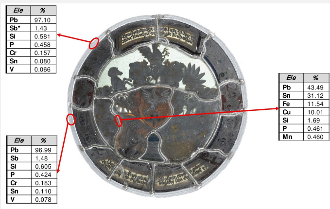
Fig. 2: XRF analysis of the different lead comes of the "Stokar" stained glass panel. Tin (Sn) content is very variable from one came to another. Those with a very low Sn but a high Sb (1.4%) contents are much more corroded,
