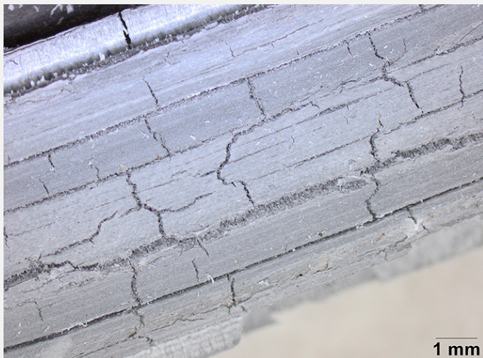
Fig. 4: Detail of the corroded lead came
