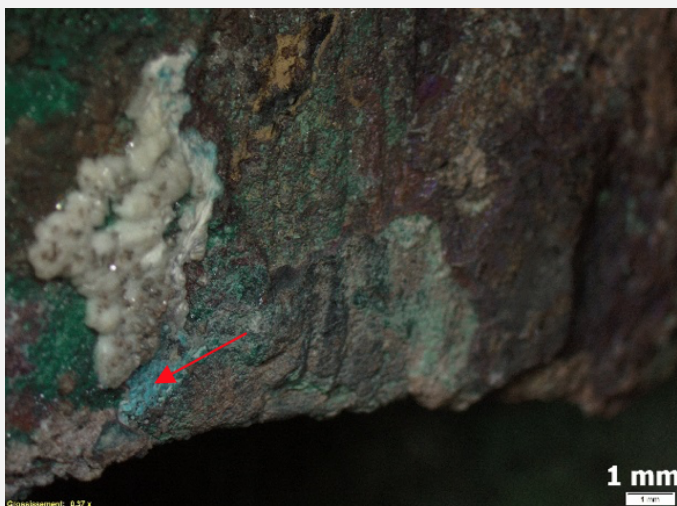
Fig. 17: Observation of the light blue corrosion product,
