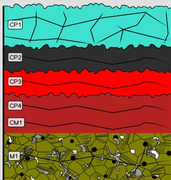
Fig. 4: Stratigraphic representation of the sample taken from the bed structure in cross-section (dark field) using the MiCorr application. The characteristics of the strata are only accessible by clicking on the drawing that redirects you to the search tool by stratigraphy representation. This representation can be compared to Fig. 8, Credit HE-Arc CR.
