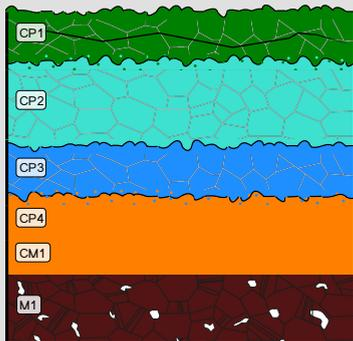
Fig. 4: Stratigraphic representation of the sample taken from the curved pin or tang in cross-section (dark field) using the MiCorr application. The characteristics of the strata are only accessible by clicking on the drawing that redirects you to the search tool by stratigraphy representation. This representation can be compared to Fig. 7, Credit HE-Arc CR.
