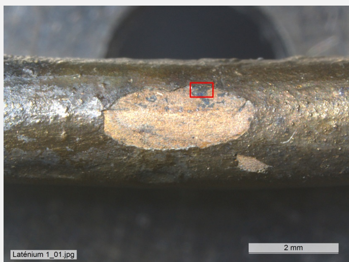
Fig. 2: Dense and smooth brown-yellow patina (detail) of the pin with lacuna showing the underlying metal with location of Fig. 4,
