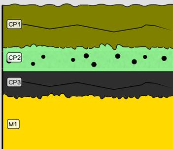
Fig. 8: Stratigraphic representation of the pin without head under binocular using the MiCorr application. The characteristics of the strata are only accessible by clicking on the drawing that redirects you to the search tool by stratigraphy representation, Credit HE-Arc CR.
