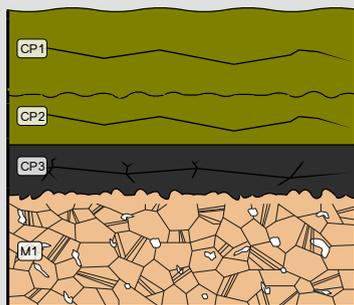
Fig. 10: Stratigraphic representation of the sample taken from the pin without head in cross-section (dark field) using the MiCorr application. The characteristics of the strata are only accessible by clicking on the drawing that redirects you to the search tool by stratigraphy representation. This representation can be compared to Fig. 16, Credit HE-Arc CR.
