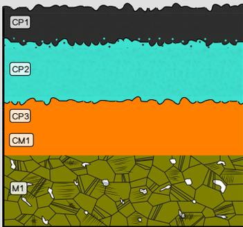
Fig. 4: Stratigraphic representation of the sample taken from the sheet fragment with dark green / grey patina in cross-section (dark field) using the MiCorr application. The characteristics of the strata are only accessible by clicking on the drawing that redirects you to the search tool by stratigraphy representation. This representation can be compared to Fig. 7, Credit HE-Arc CR.
